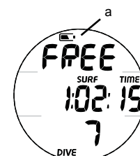
Fig. 2 - LOW BATTERY WARNING
