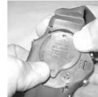
Fig. 74B - COVER INSTALLATION (without tool)
