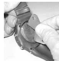
Fig. 70A - BATTERY COVER REMOVAL (using tool)
