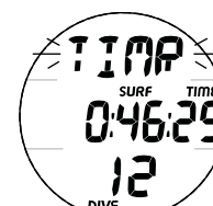
Fig. 61 - FREE SURFACE CDT ALARM
