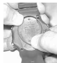
Fig. 70B - BATTERY COVER REMOVAL (without tool)
